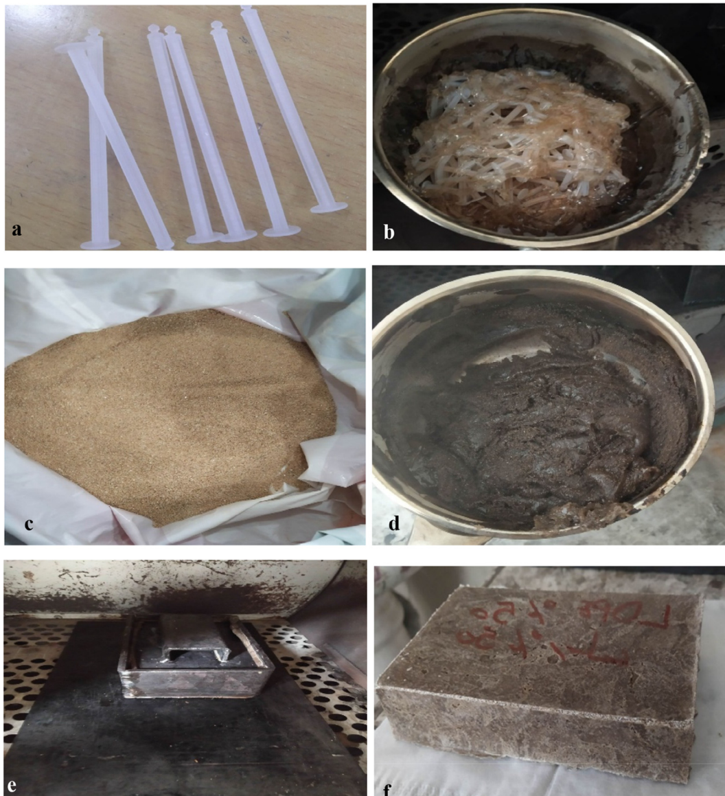
Fig. 1. a) LDPE waste material, b) Melting of low density polyethylene in a closed furnace, c) Filler (sand or sawdust) sieved and required amount measured, d) Homogeneous mixing of molten LDPE with the filler, e) Pour the sample into the mould and leave to harden; and f) The sample removed from the mould to produce a brick sample.
