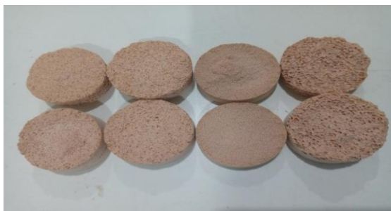
Figure 1. Porous geopolymer samples with different porosity
