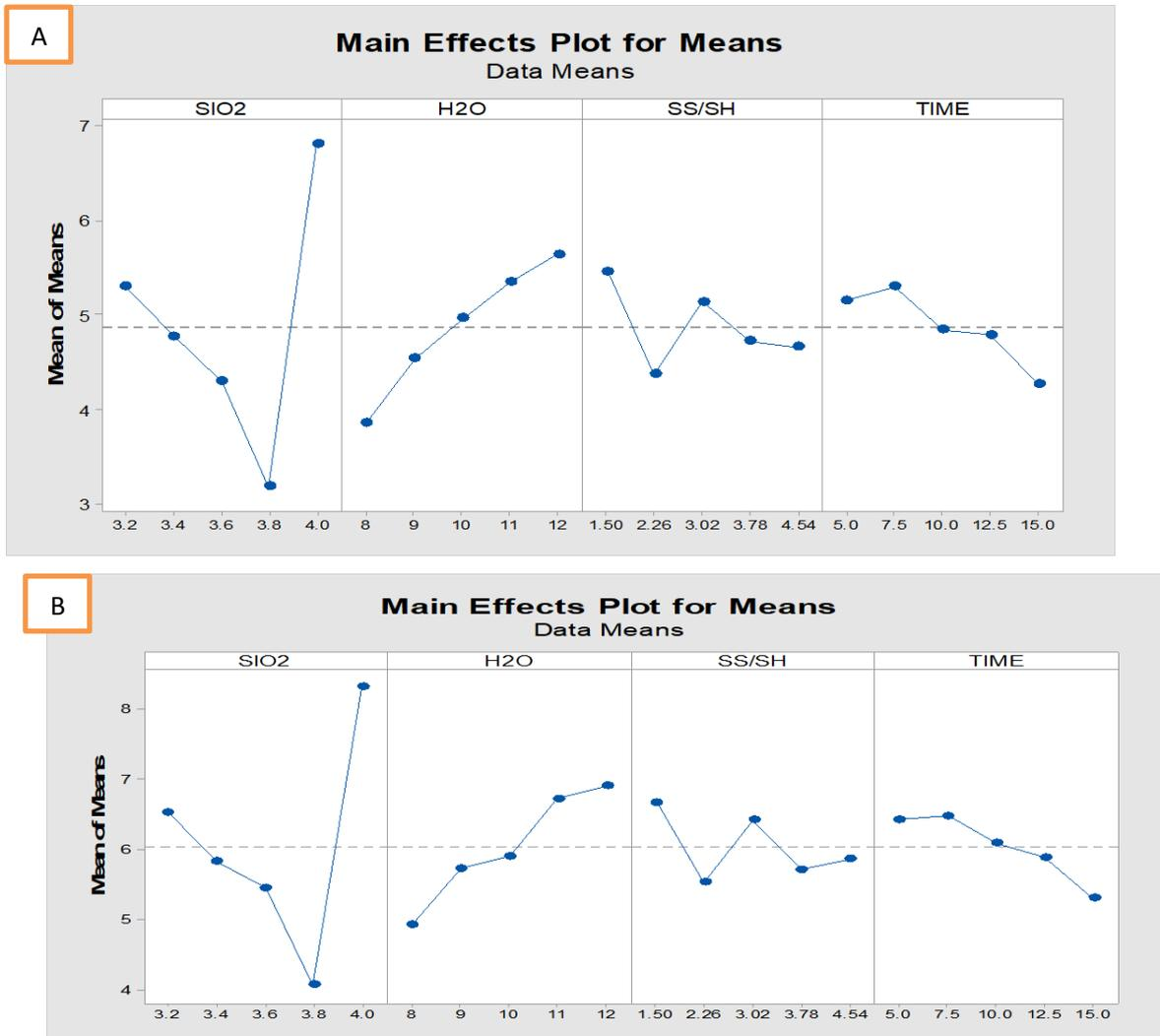
**Figure 8.** (A) initial setting time and (B) the final setting time of Geopolymer batch GP1
