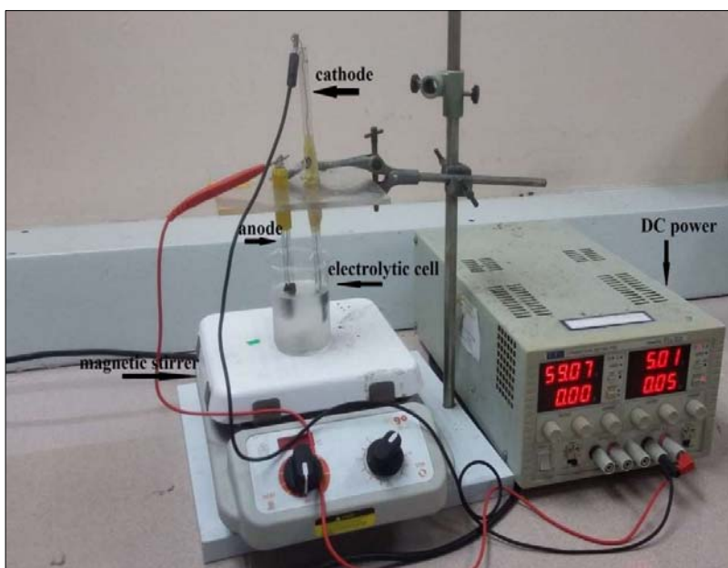
Figure 3. The schematic diagram of the electrochemical process
