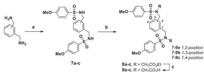
Scheme 1. Synthesis of disubstituted xylylene derivatives **9a-c**.<sup>a</sup> Reagents and conditions: (a) 4-methoxybenzenesulfonyl chloride, TEA, DCM, rt, overnight, 75–82%; (b) ethyl 2-bromoacetate,  $K_2CO_3$ , DMF, rt, overnight, 80–87%; (c) NaOH, EtOH,  $H_2O$ , rt, 72–80%.
