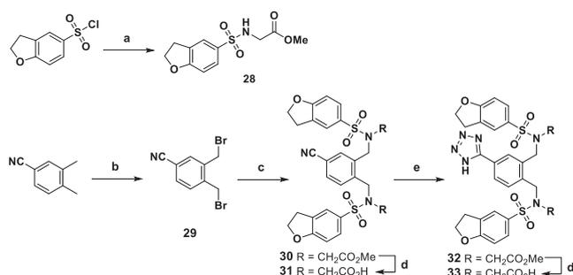
**Scheme 6.** Synthesis of compounds **31** and **33**<sup>a</sup>. <sup>a</sup>Reagents and conditions: (a) glycine methyl ester HCl, TEA, DCM, rt, overnight, 80%; (b) NBS, AIBN, CH<sub>2</sub>Cl<sub>2</sub>, 75 °C, overnight, 84%; (c) **28**, K<sub>2</sub>CO<sub>3</sub>, DMF, rt, overnight, 82%; (d) NaOH, EtOH, H<sub>2</sub>O, rt, 74–84%; (e) NaN<sub>3</sub>, NH<sub>4</sub>Cl, DMF, 85 °C, overnight, 72%.
