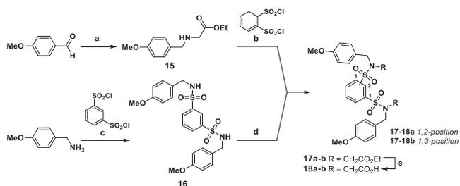
**Scheme 3.** Synthesis of compounds **18a-b**<sup>a</sup>. <sup>a</sup>Reagents and conditions: (a) ethyl glycinate HCl, NaBH<sub>3</sub>CN, EtOH, rt, overnight, 51%; (b) K<sub>2</sub>CO<sub>3</sub>, DMF, rt, overnight, 71%; (c) TEA, DCM, rt, overnight, 81%; (d) ethyl 2-bromoacetate, K<sub>2</sub>CO<sub>3</sub>, DMF, rt, overnight, 79%; (e) NaOH, EtOH, H<sub>2</sub>O, rt, 87%.
