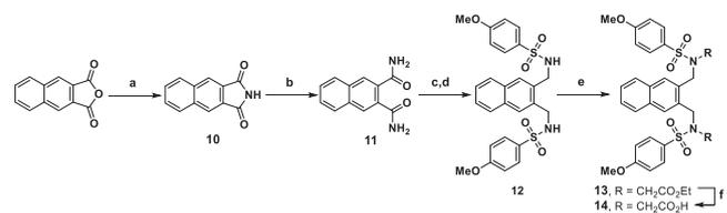
Scheme 2. Synthesis of 1,2-disubstituted naphthalene derivative **14**.<sup>a</sup> Reagents and conditions: (a) Urea, 170 °C (microwave), 2 h, 90%; (b)  $NH_3$ , DMF, rt to 50 °C, 8 h, 67%; (c)  $BH_3 \cdot Me_2S$  complex, THF, reflux, 2 d, 63%; (d) 4-methoxybenzenesulfonyl chloride, TEA, DCM, rt, overnight, 63%; (e) ethyl 2-bromoacetate,  $K_2CO_3$ , DMF, rt, overnight, 87%; (f) NaOH, EtOH,  $H_2O$ , rt, 79%.
