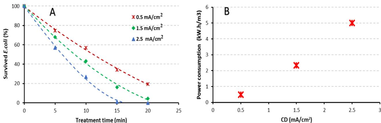
Fig. 5. Effect of ES on: (A) *E. coli* inactivation, (B) Power consumption.
