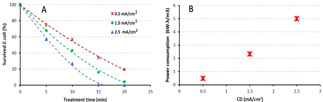
Fig. 4. Effect of CD on: (A) *E. coli* inactivation, (B) Power consumption.
