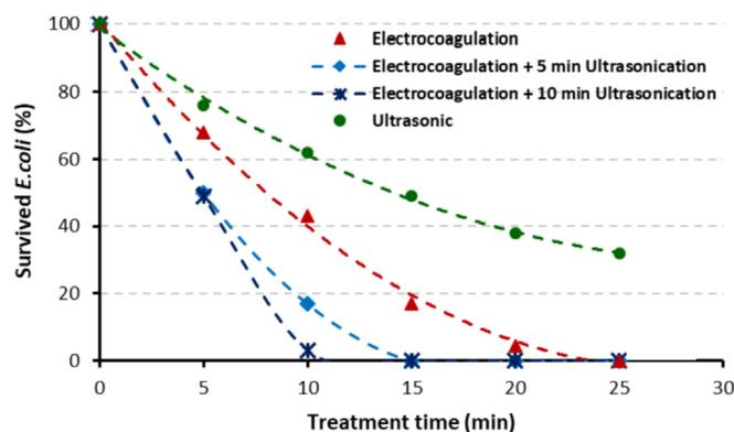
Fig. 6. Influence of ultrasonic field on *E. coli* inactivation.
