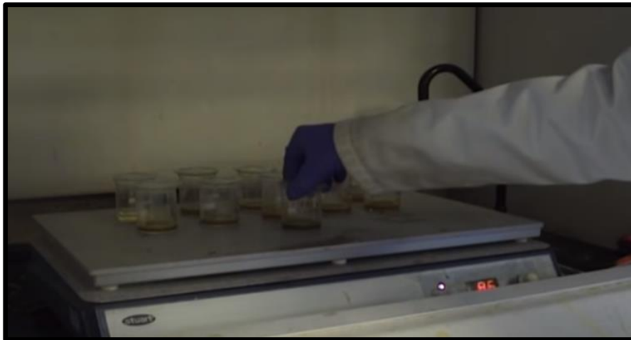
Figure 2. putting the samples on the hot plate for digestion process
