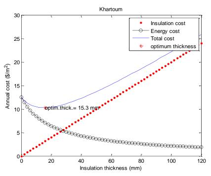
**Fig. 2.** Effect of the insulation thickness of extruded polystyrene (XPS) on the total cost in case cooling energy requirement used perforated red brick in Khartoum
