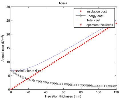
**Fig. 5.** Effect of the insulation thickness of extruded polystyrene (XPS) on the total cost in case cooling energy requirement used perforated red brick in Nyala
