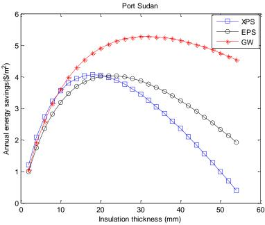
**Fig. 8.** Comparison of the annual energy savings of all insulation materials in the case of the cooling requirement for selected fired clay bricks in Port Sudan
