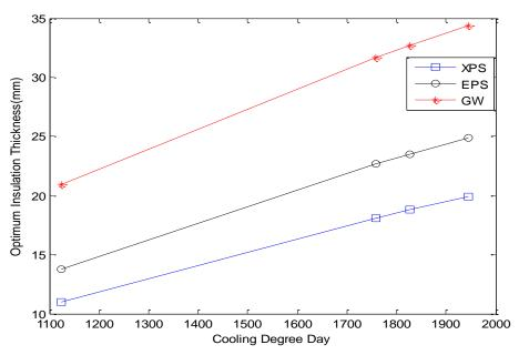
**Fig. 10.** Optimum insulation thicknesses of external walls versus cooling degree days (CDD) values for three insulation materials for all considered cities
