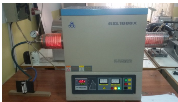
Figure 3. The GSL-1600-60X vacuum tube furnace used in this work
